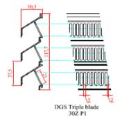
Cross section of the 30Z P1 blade with 2.5mm X 21mm insect punchings at "C"
