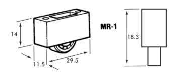
The MR 1 secondary glazing roller has 16mm (5/8") diameter steel flat roller bearing set into a black plastic carriage incorporating two No, 3mm fixing holes that are suitable for No 4 installation screws.
